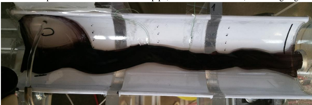
Run c: hit point at opposite side of the nozzle, flow rate ca. 7 L/min, low swing angle
