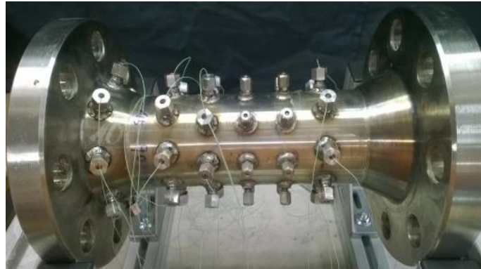
Figure 2-16: With micro-thermocouple equipped thermocouple (TC)-module
