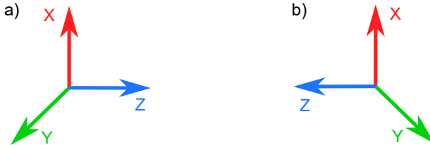
Figure 5.1: Representations of a Cartesian right-handed basis (a) as well as a left-handed basis (b).
