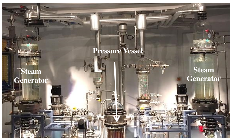
Figure 2-1: PWR glass model at GfS, Essen [65]
