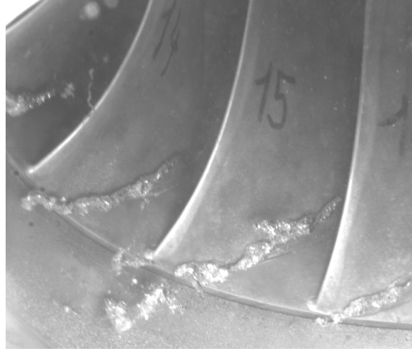
b) Inter-blade vortices at deep part load.
