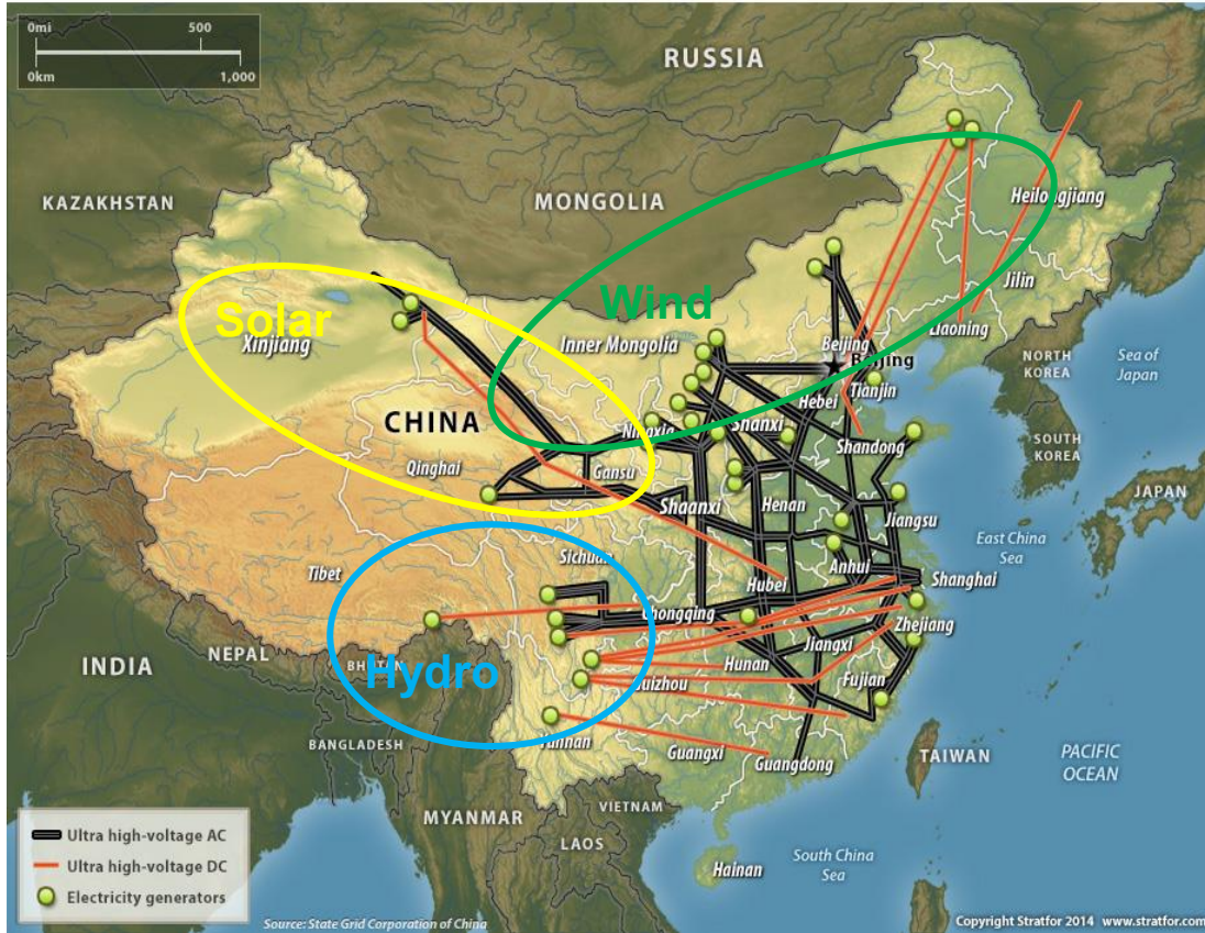
Figure 5.5 China's national power grid plan for 2020 (map source: State Grid Corporation of China).
