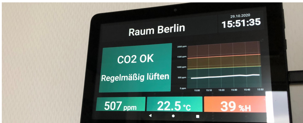
Figure 5.1: Grafana visualization of the IoT Data gathered in a SPIRIT/21 meeting room
