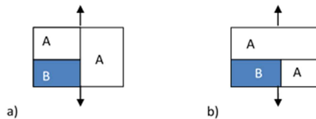
Figure 4-A2: Schematic representation of the consequence of calculation of Young's modulus. a) First the left part of the cell is calculated according to the formula by Reuss and after that the whole cell is calculated with the Voigt's formula; b) First the lower part of the composite is calculated with the Voigt's formula and then the Young's modulus of the specimen is calculated with the formula by Reuss [43]
