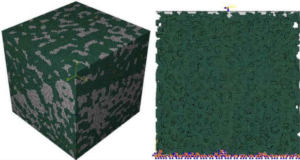
Figure 10-8: Left- The final result of the procedure to create a voxelmodel: Green represents the calcium material, white is air, which is deleted before using the mesh in the Finite Element analysis to avoid high amounts of elements.Right: The boundary conditions used in the FEM-simulation: An Analytic Rigid (a not mesh able part in ABAQUS) is used to transfer the force through a Rigid Body Constraint. The bottom part is fixed through the boundary conditions
