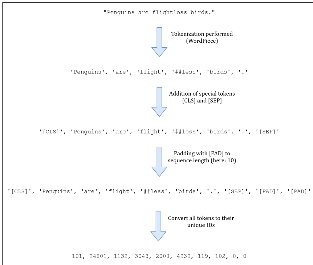
Figure A.1: Pre-processing steps for input sequences in BERT applied to an example sentence [DCLT19]
