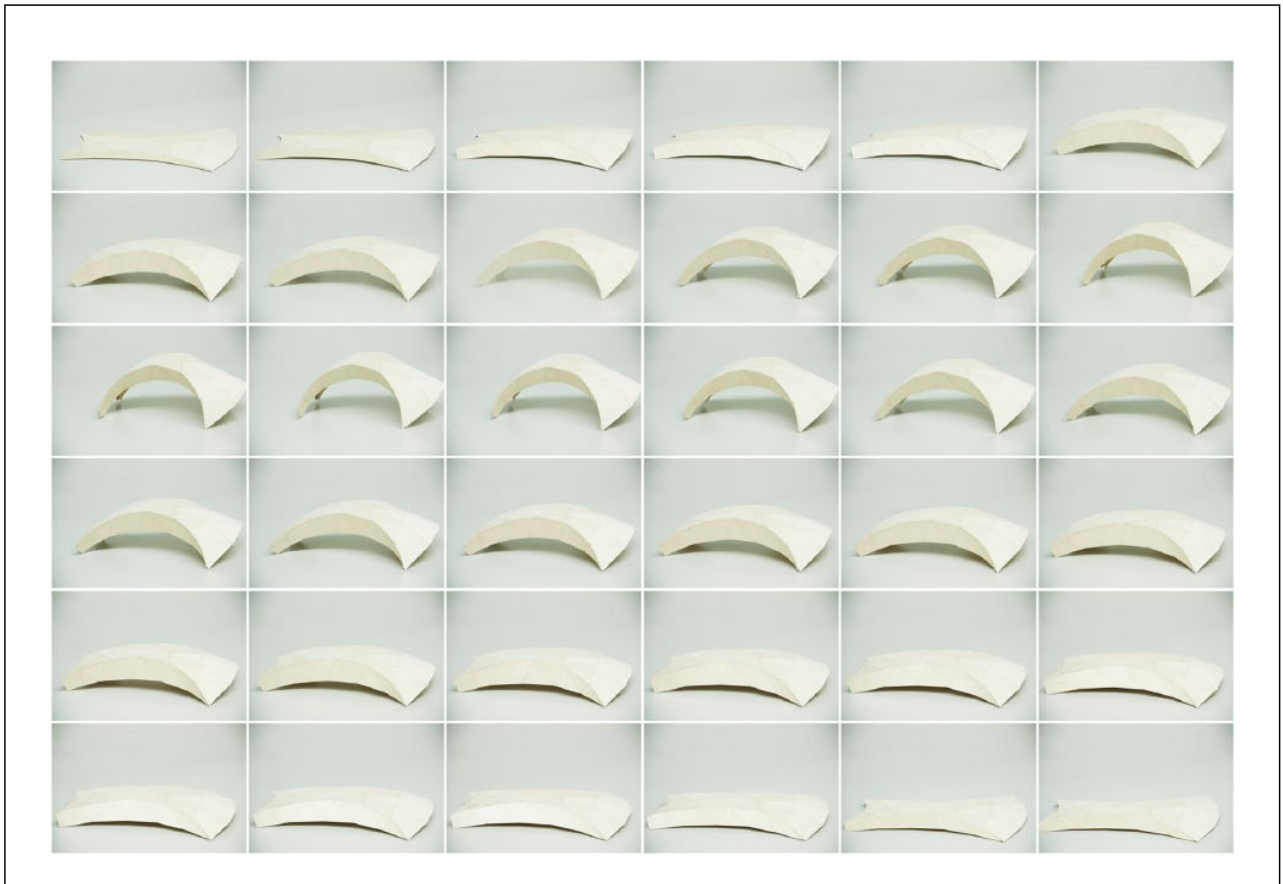
Figure 4. Self-forming and self-rigidizing responsive veneer surfaces.
