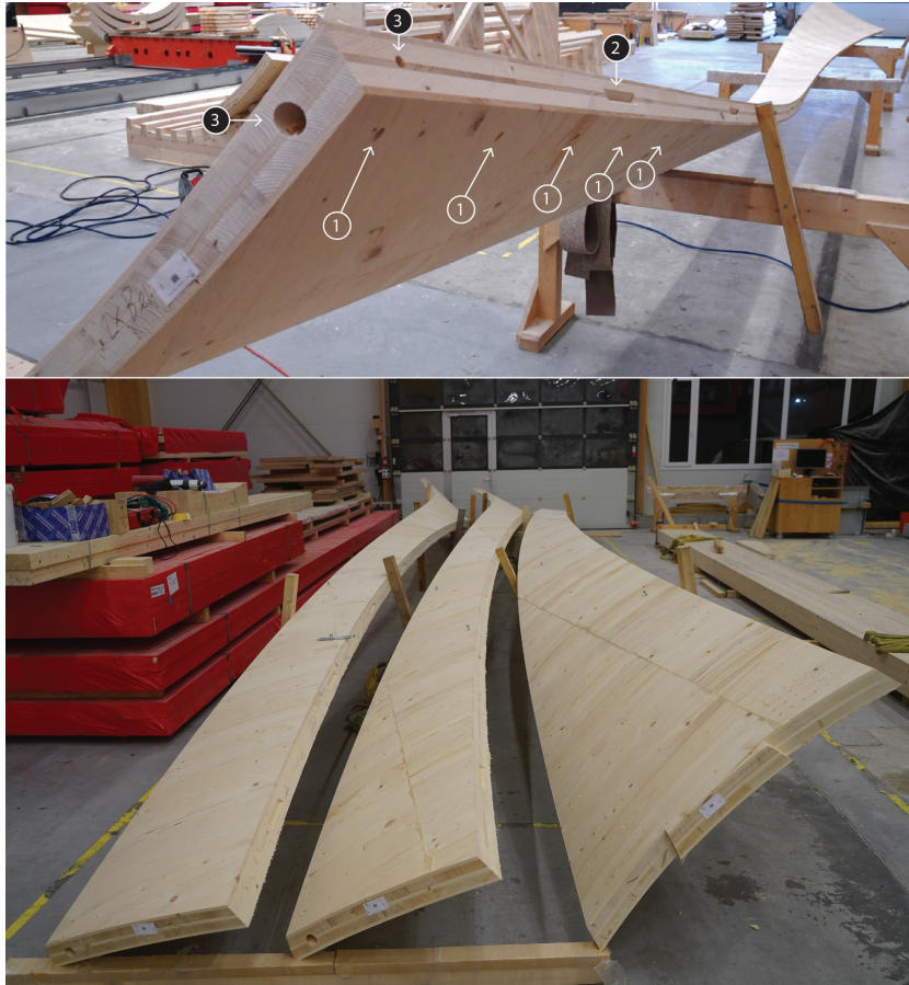
Figure 6.8: Completed self-shaped CLT components for the Urbach Tower. Top: Close-up of the CNC detailing. (1) Pre-drilled holes for crossing screws used for onsite connection of assembly groups from the interior, 12 mm face drill hole and 3 mm pre-drill hole for 6 mm diameter 120 mm long fully threaded stainless-steel screw, variable spacing based on loading. (2) Cutout for placement of square cross-section hardwood alignment block, 19.5 x 19.5 x 150 mm spaced ca. 1200 mm). (3) Holes for connection and storage of fabric strap for lifting during assembly and planned disassembly onsite. Bottom: Three completed components prior to assembly into groups
