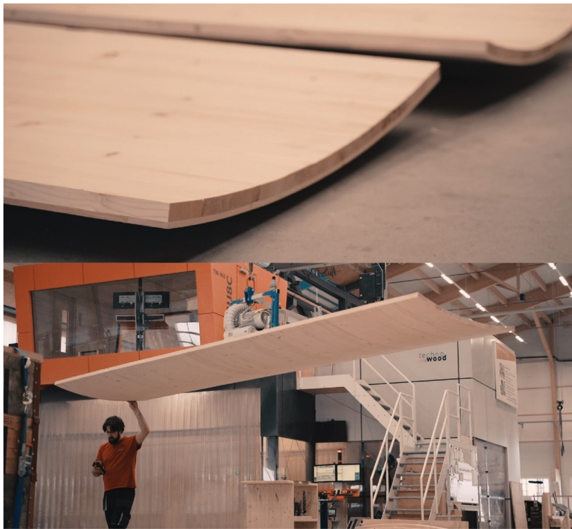
Figure 6.5: Curved wood bilayers displaying the added stiffness resulting from the curvature. Top: suspended from a central point for transport in the production hall. Bottom: suspended along the longitudinal axis for measurement.
