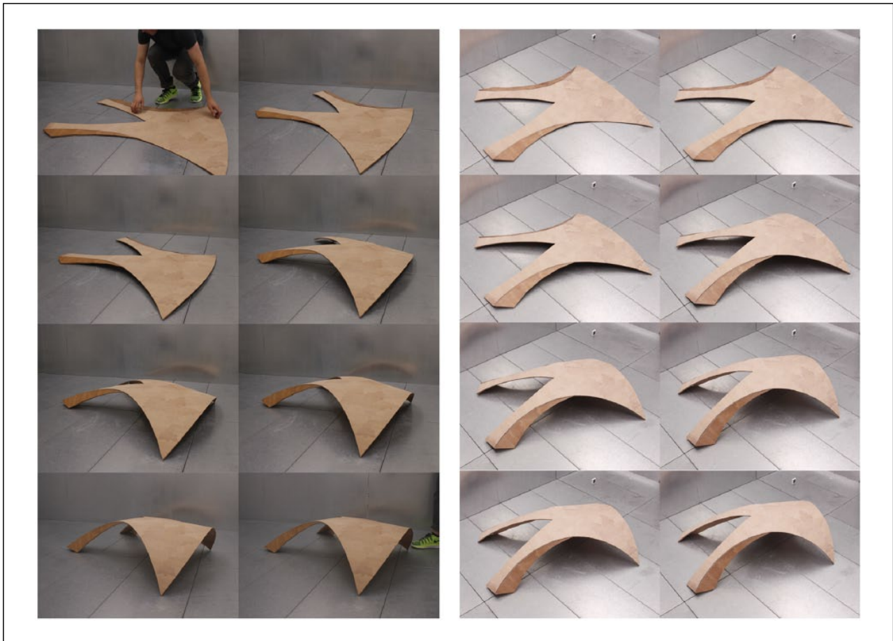
Figure 6. Self-constructing and self-rigidizing responsive timber composite surfaces, 2 views.
