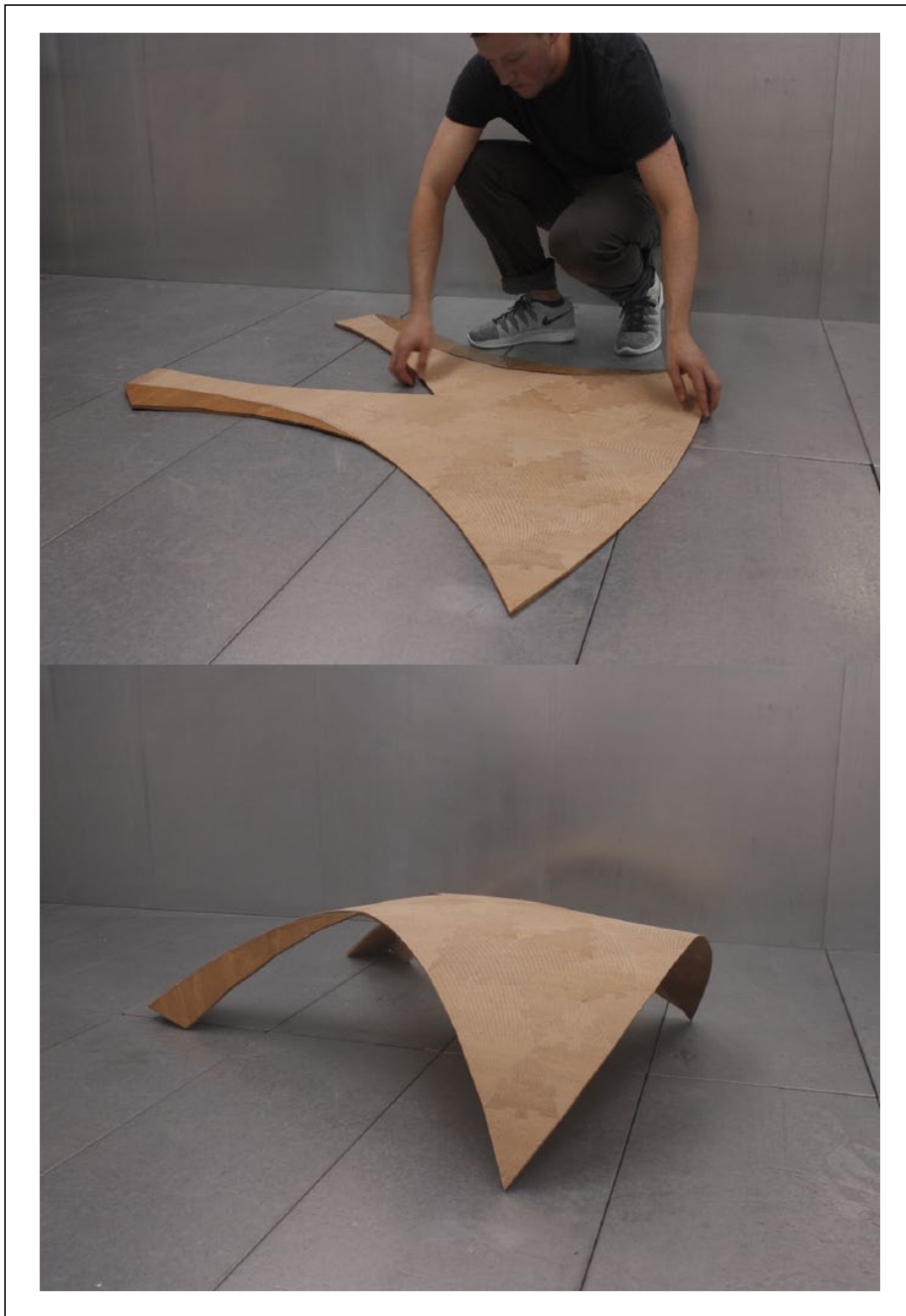
Figure 1. Self-constructing timber surface in a flat and a fully actuated three-dimensional state.
