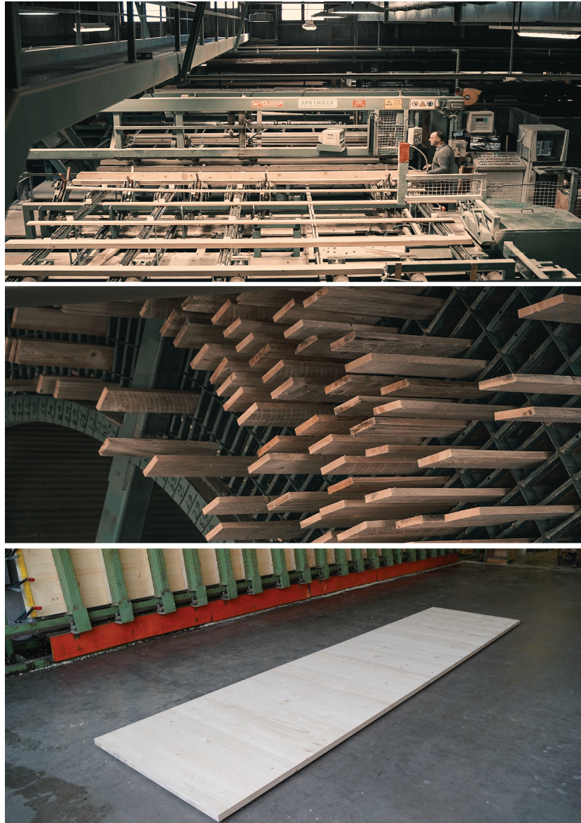
Figure 6.3: Sorting of boards on the sawmill production line. Top: Standard grading and inline measurement of WMC. Middle: Semi-automatic sorting and collection of the boards in the sorting wheel. Bottom: Assembly and flat pressing of the selected boards into bilayer plates.
