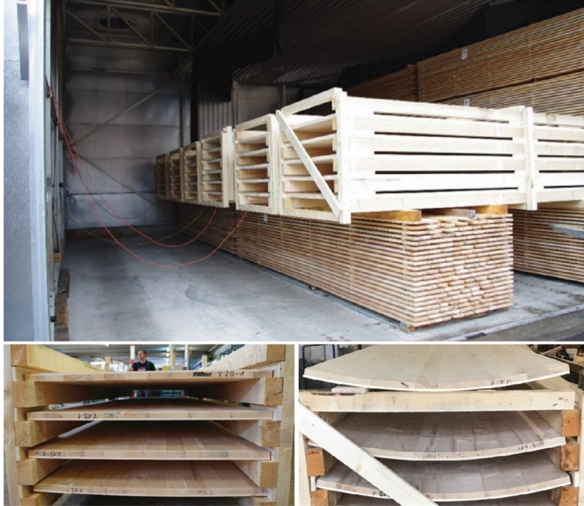
Figure 6.4: Kiln-drying of the spruce-wood bilayers. Top: Bilayer racks being loaded into the drying kiln with other stacks and sensors installed for monitoring WMC. Bottom left and right: The flat bilayers with a high WMC before drying, and curved bilayers with a low WMC after drying
