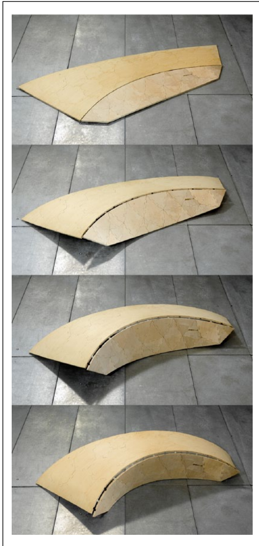
Figure 7. Self-constructing and self-rigidizing responsive timber surfaces.
