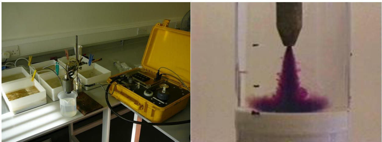
Figure 8: CSM measurements within estuarine biofilm grown in boxes on glass beads. Left: the test or erosion chamber (grey) in idle position above the beaker is connected to the yellow suitcase containing air supply and water bottles for the perpendicular water jets as well as the digital panel and keypad for the various erosion programs to apply and measure. Right: visualization of one CSM jet within the test chamber by applying a potassium permanganate solution (Image from SERG lab of Prof. D.M. Paterson).
