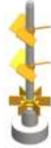
FIGURE E.2: Schematic illustration of two A340 and one rushton impeller representing impeller setup 2.
