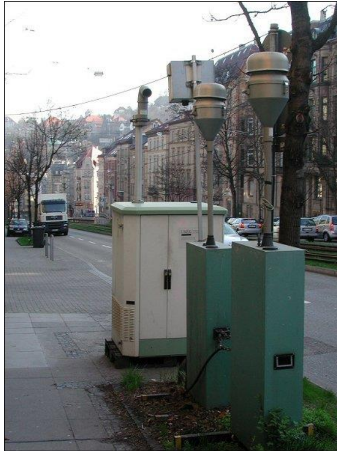
Figure 3.1. Particulate Sampler MicroPNS Type LVS close to a LUBW Station in Hohenheimer Straße (Stuttgart).
