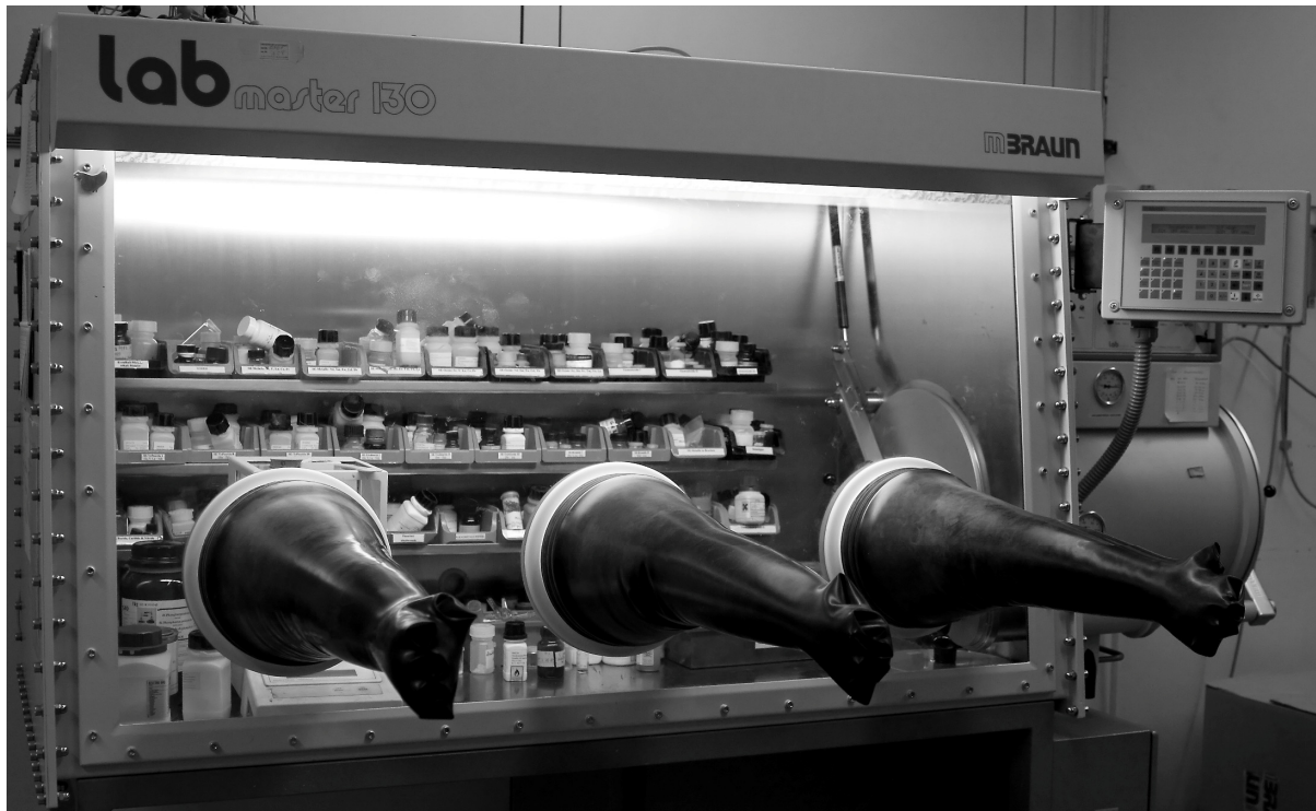
Abb. 2.1.2.a: Argon-Glove-Box Labmaster MB 130 (Firma MBRAUN, Garching).
