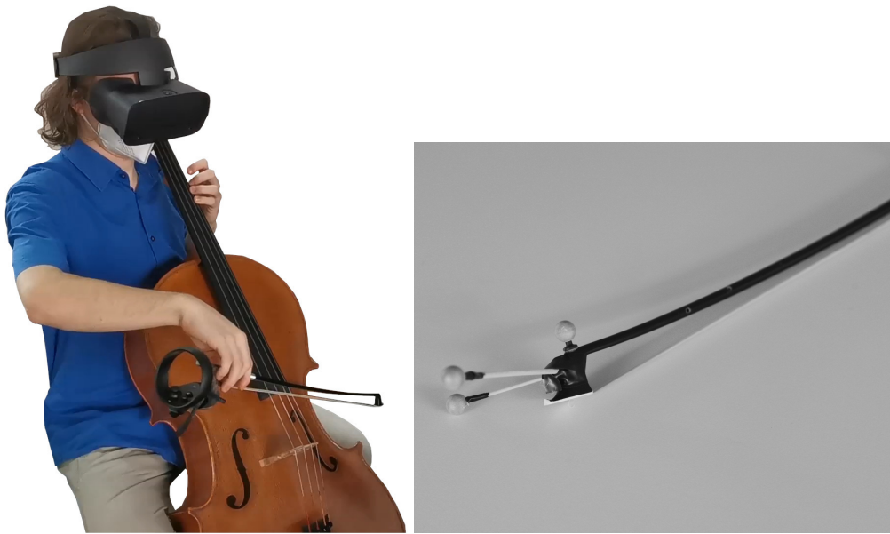
(a) As a cheap and easy solution, we taped a VR controller to the bow. The controller is then tracked by the five built-in cameras of the HMD. Image from our previously published paper [HKT+22]. (b) Later, we used the OptiTrack system to capture the motion of the bow. The gray spheres are infrared-reflective markers that are tracked by eight cameras distributed around the room.
