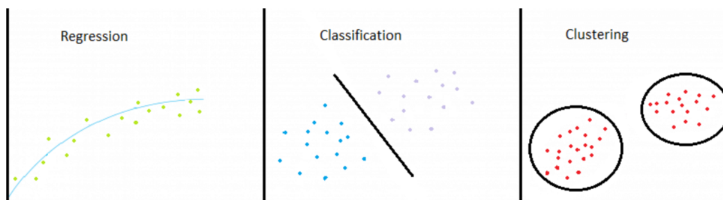
Figure 2.1: Left: A regression problem. Middle: A classification problem with 2 classes. Right: A clustering problem with 2 clusters.
