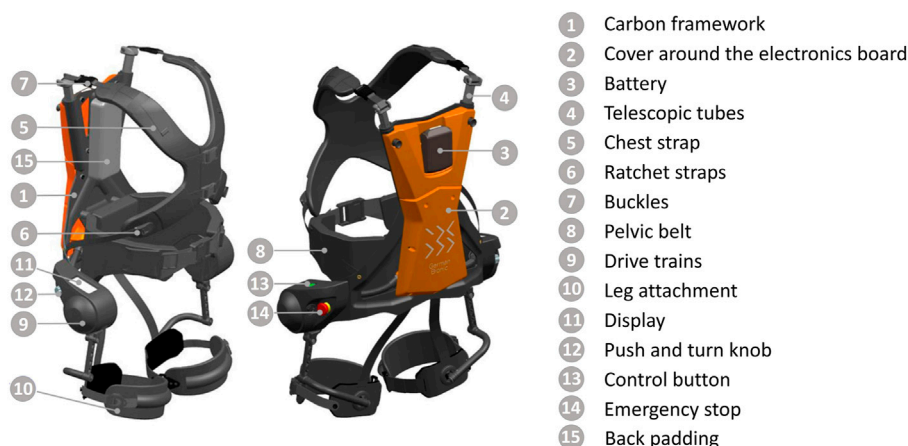
FIGURE 1 Labelled 3D model of the active exoskeleton Cray X in its fourth generation (German Bionic Systems GmbH, Germany).
