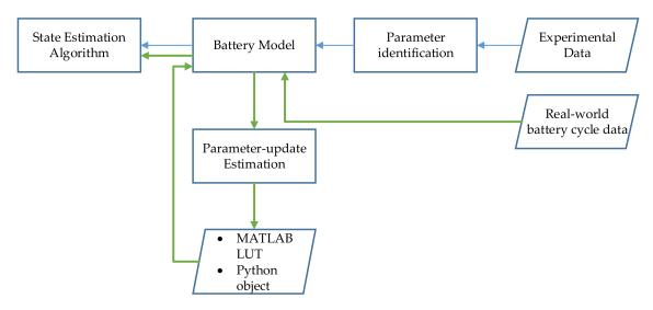
Figure 3. Software segment for implementation steps.
