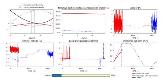
Figure 5. Comparison between output parameters of two discharge characteristics.
