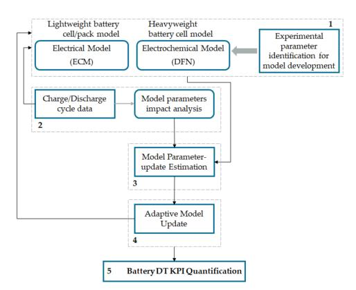
Figure 2. Approach for battery DT implementation.
