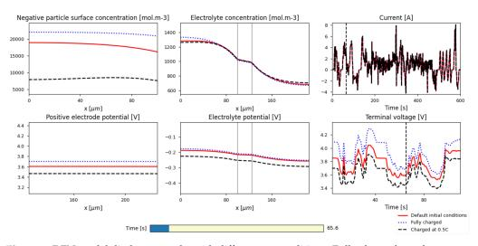
**Figure 4.** DFN model discharge results with different preconditions. Fully charged—code statement (2). Complete discharge and slow charge—code statement (3).
