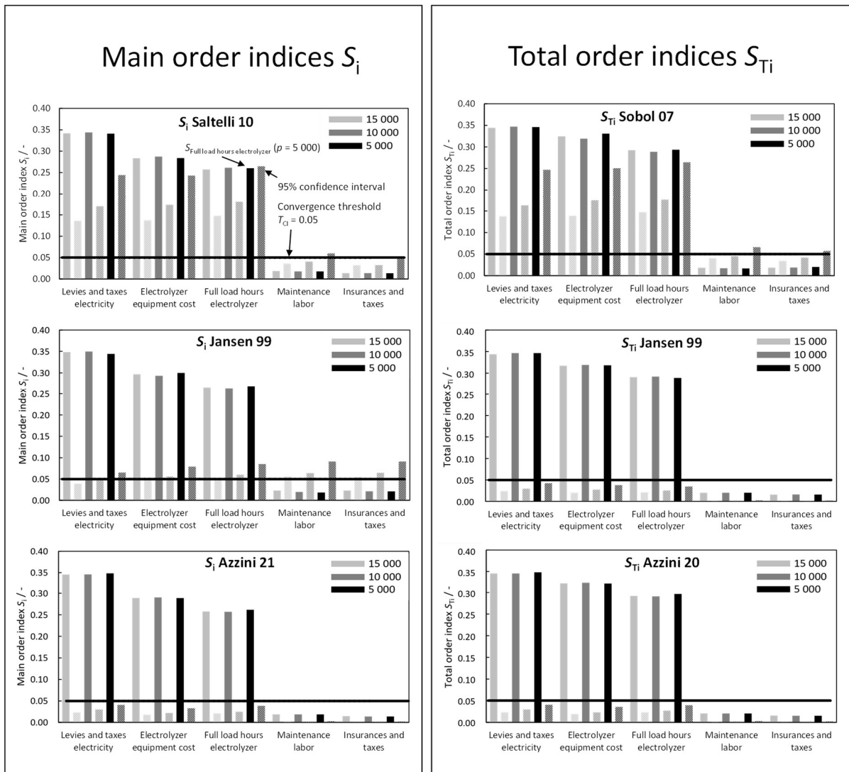
Figure 12: Main and total effect indices at varying sample sizes (model evaluations) as well as the respective 95 % confidence intervals (bootstrapping sample size equals sampling size for calculating S_i/S_{Ti} , number of re-evaluations for bootstrapping is 1 000). The threshold for stochastic convergence is assumed to be T_{CI} = 0.05 (reproduced from Paper 3).
