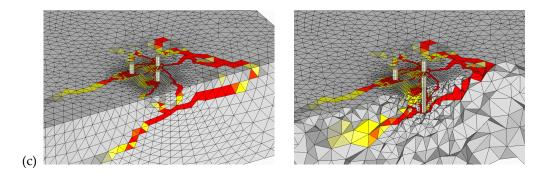
**Figure 10.** Crack pattern obtained from numerical analysis for Group Tri-B loaded parallel to the edge (a) first cracks, (b) at peak load, and (c) post-peak phase.
