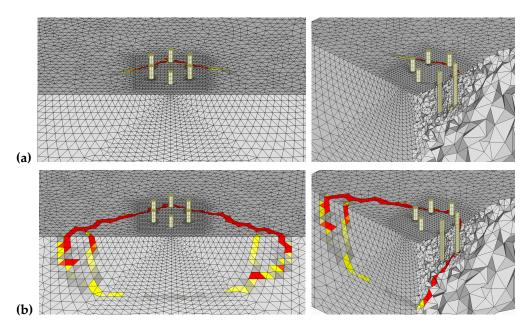
**Figure 14.** Crack pattern obtained from numerical analysis for Group Hex-B (a) at peak load, and (b) Crack pattern in the post-peak phase.
