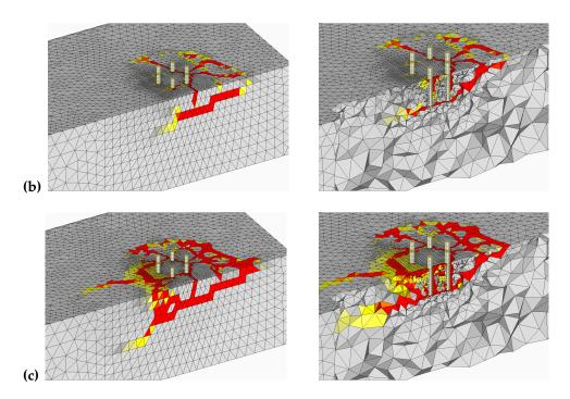
**Figure 13.** Crack pattern obtained from numerical analysis for Group Hex-A loaded parallel to the edge (a) first cracks, (b) at peak load, and (c) post-peak phase.
