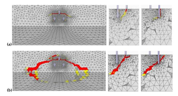
**Figure 7.** Crack pattern obtained from numerical analysis for Group Tri-A loaded perpendicular to the edge (a) at peak load, and (b) in post-peak phase.
