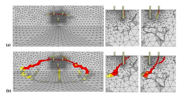
**Figure 9.** Crack pattern obtained from numerical analysis for Group Tri-B loaded perpendicular to the edge (a) at peak load, and (b) post-peak phase.
