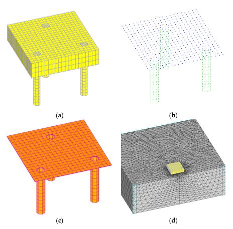
**Figure 4.** (a) 3D finite element model of GS-Tri-A, (b) base plate and anchos, (c) contact between anchor and concrete and contact between the base plate and concrete surface, (d) bond type bar elements along the anchor shaft and contact type bar elements below the base plate.
