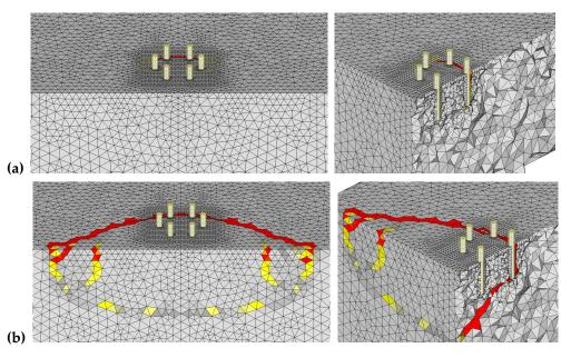
**Figure 12.** Crack pattern obtained from numerical analysis for Group Hex-A (**a**) at peak load, and (**b**) Crack pattern in the post-peak phase.
