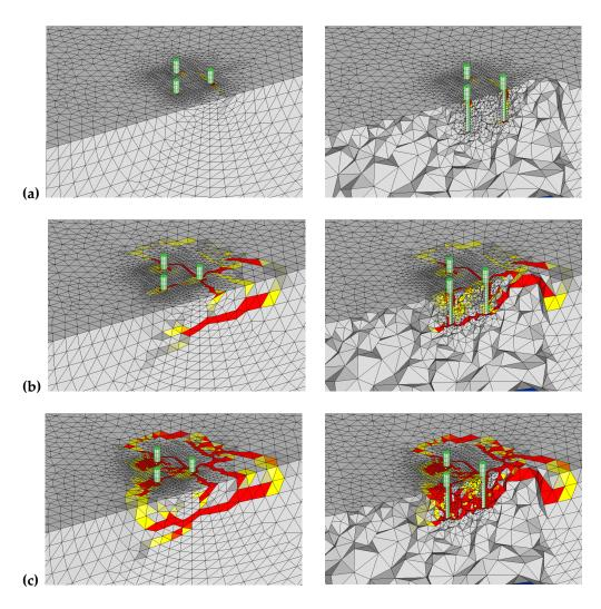
**Figure 8.** Crack pattern obtained from numerical analysis for Group Tri-A loaded parallel to the edge (a) first cracks, (b) at peak load, and (c) post-peak phase.
