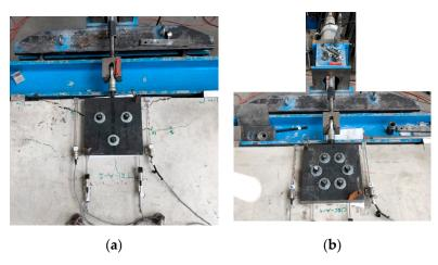
**Figure 2.** Test setup used by Bokor et al. [12] for conducting shear tests on anchorages of (a) triangular configuration and (b) hexagonal configuration (photos by author).
