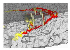
**Figure 15.** Crack pattern obtained from numerical analysis for Group Hex-B loaded parallel to the edge (**a**) first cracks, (**b**) at peak load, and (**c**) post-peak phase.
