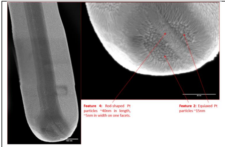
Figure A.11 Close up of the Au-Pt NW tip with an embedded twin. Scale bars are 100 nm (left) and 50 nm (right). SEM images.
