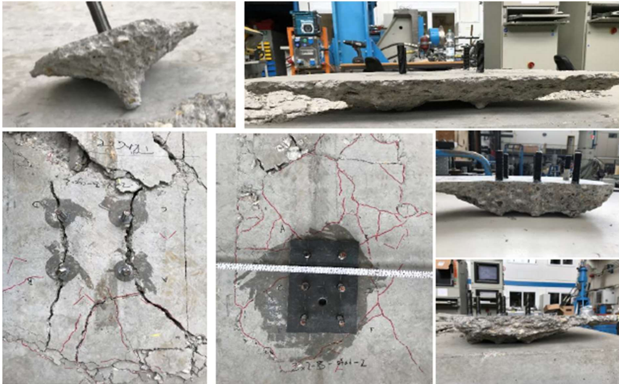
Figure 8.3. Typical failure modes obtained from monotonic and cyclic tension tests.
