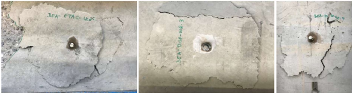
Figure 5.18. Typical failure modes of bonded expansion anchors in uncracked and cracked concrete.
