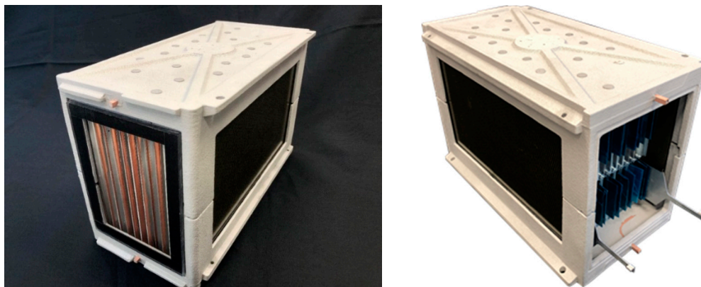
Figure 10. Demonstrator of the battery module. Left: rear view with window to provide insight into the module. Right: front view with stacked battery pouch cells and without cover.
