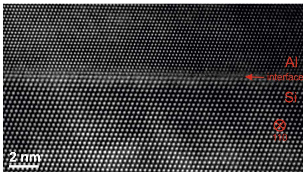
Fig. 3.3. HRTEM image of the Al/Si interface revealing that the interface is atomically sharp.
