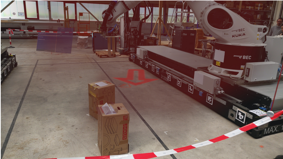
Figure 5.2: Picture taken with the HoloLens while running the study software. The Safety Bubble visualization is visible and in the background is the VIZOR interface by Yang et al. [32] the human user has to interact with. The red sphere surrounding the user (hardly visible) and the red arrow are projected in the middle of the picture.
