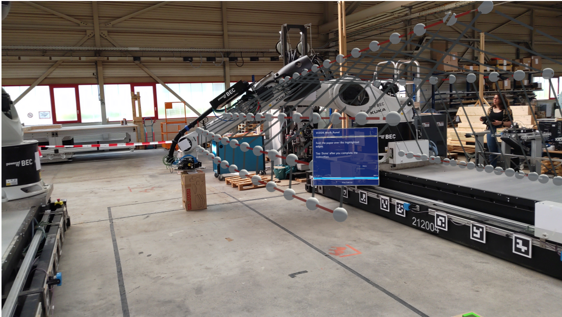
Figure 5.1: Picture taken with the HoloLens while running the study software. The trajectory visualization is visible and in front is the VIZOR interface by Yang et al. [32] the human user has to interact with. The white spheres represent the joints of the robot and are connected through the gray lines to represent the robot's position at a given time step. The red lines show the movement of a single joint.
