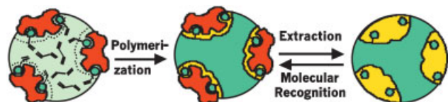
Figure 1. General scheme for the preparation of molecularly imprinted nanospheres and their use for molecular recognition: Template molecules induce the formation of binding sites during the miniemulsion polymerisation. The templates are extracted from the highly cross-linked particles and are molecularly recognised by the nanospheres selective binding sites.
