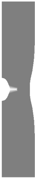
Fig. 4.74(a): Crack propagation in the flat tensile specimen (nonlocal model), contour plot of damage
