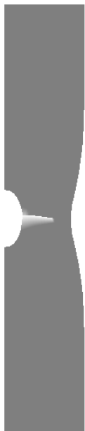
Fig. 4.73(a): Crack propagation in the flat tensile specimen (local model), contour plot damage
