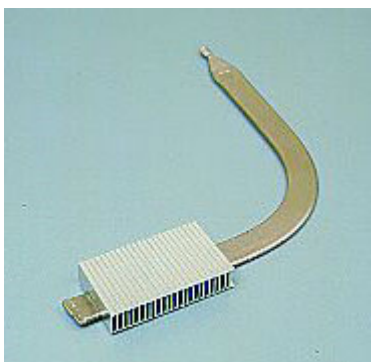
Fig. 3.2: Example of high-efficiency micro-heat pipe application (heater block dimensions: 5 \times 20 \times 35 \text{ mm} )
