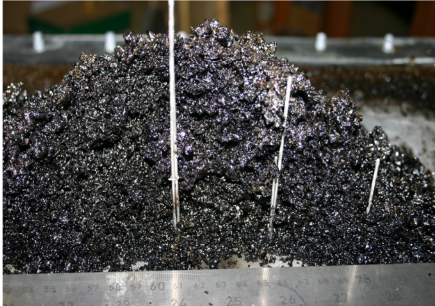
Figure 1.3: Debris bed from DEFOR 07 experiments [40].
