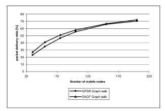
Figure 7. Packet Delivery Ratio with GPSR and SAGF in graph walk model
