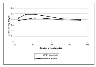
Figure 9. Packet Delivery Delay with GPSR and SAGF in graph walk model
