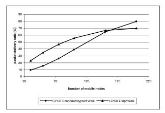
Figure 6. Packet Delivery Ratio of GPSR in random waypoint and graph walk models
