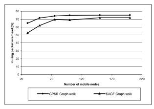
Figure 10. Routing Packet Overhead with GPSR and SAGF in graph walk model
