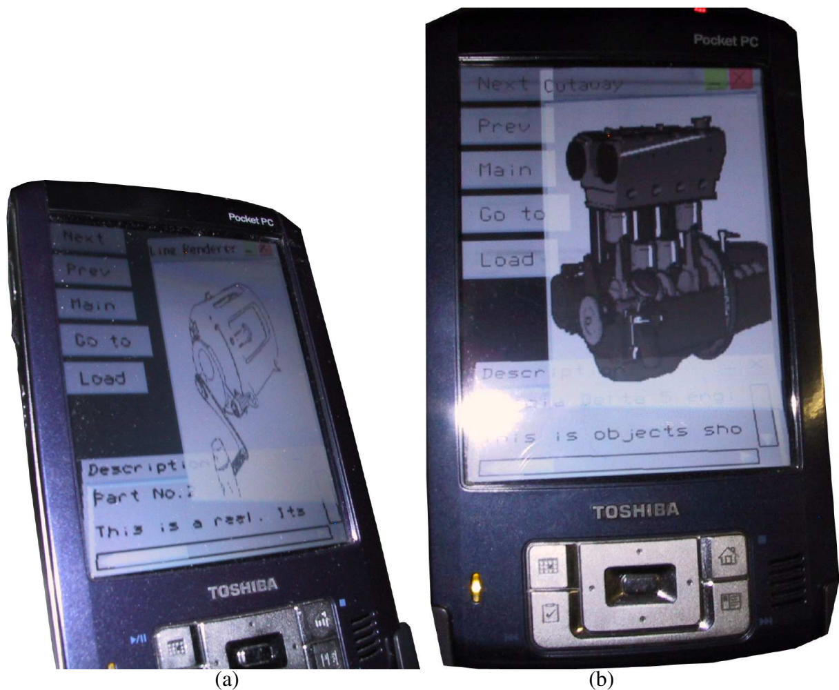
Figure 6.2: Two example applications running on a PocketPC using a combination of different methods described in this thesis. (a) Line rendering running in a window of the 3D GUI. (b) Image-based remote rendering in a window of the 3D GUI rendering a cutaway view of the Lancia Delta 5 engine.
