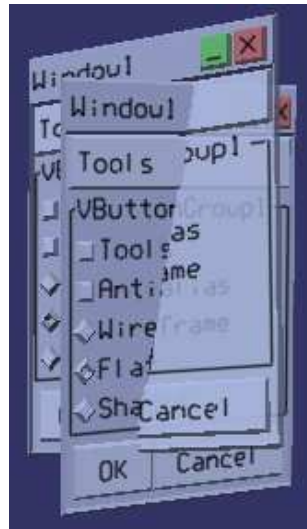
Figure 5.4: Overlapping and occlusion of windows when standard depth test is used in a 3D windowing system.
