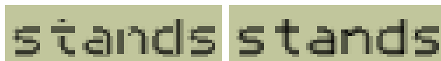
Figure 5.6: Antialiasing of lines using GL_LINE_SMOOTH option for font output with (left) depth protection and (right) without depth protection.
