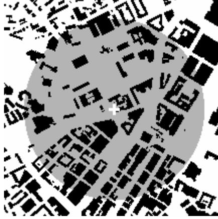
Figure 4.1: Communication area of a WLAN node computed with the free space model
