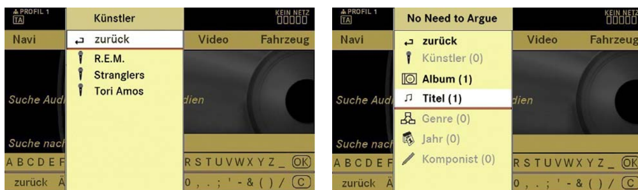
Figure 5.3: Category-free search – multiple results within one category (left); resolution proposal for multiple results in different categories (right)
