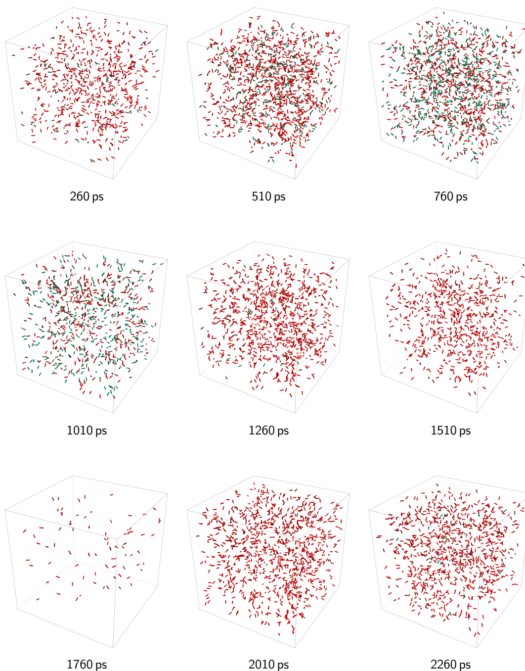
Figure 4.4: Rendering of atoms' displacement field. Here, a time window of only one frame was used to compute the displacement field for all atom types using averaged atom positions (25 frames). Several pulsating peaks can be observed right at the beginning of the time series. Starting at about 6000 ps the atoms are becoming more mobile. Their mobility further increases until the end of the time series is reached.
