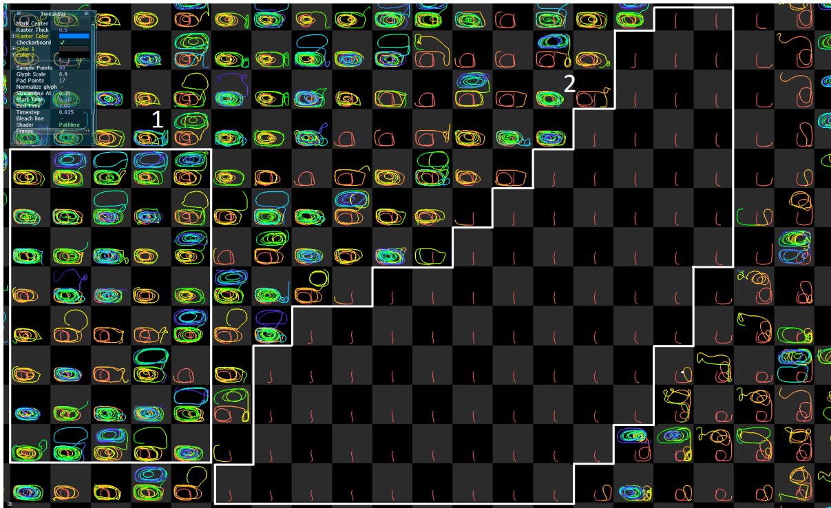
Figure 5.3: zoomed-in view on area 2 from Fig.4.7. Region 1 shows a region where all pathlines are different from each other. Note the big difference between adjacent pathlines. They do have in common that they mostly stay in the lower half, but still some pathlines have a short stay in the upper half and a few of them curl in the upper half until the end of time range(4 pathlines in the top row). Region 2 marks the region of pathlines ending up at the edge of the domain.
