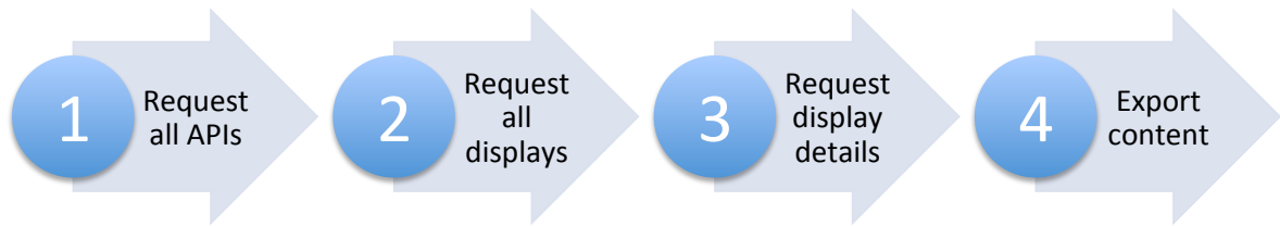
Figure 4.6: Example of an API access flow: first the client can access the API root (1) that provides links to each API resource. An API resource then lists all instances (2) and provides links to the detail page for each listed instance (3), which then contains links to other possible APIs, e.g. exporting the display content (4).
