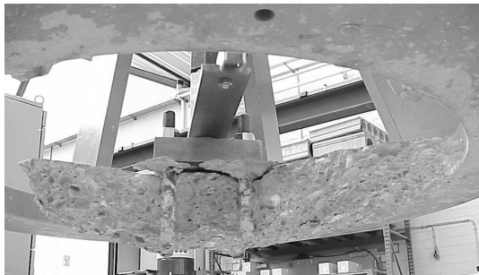
a) M16, h_{ef} = 80 \text{ mm} , \tau_u \sim 6,0 \text{ N/mm}^2 , Mörtel WW
