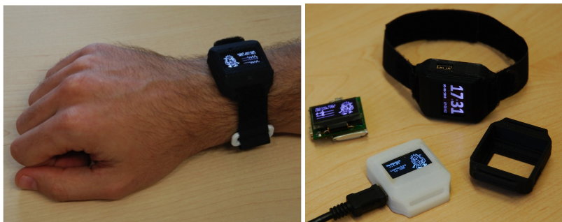
Figure 5.4: HedgeHog is a device worn like an actigraph at the dominant wrist records motion, posture, and light data over a long time-span.
