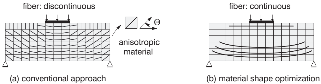
Figure 1.4: Concept of material shape optimization , (a) conventional approach for fiber orientation and (b) material shape optimization
