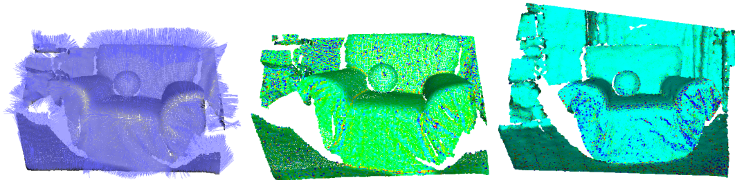
Fig. 22: From left to right: image with the calculated normals, image with the mean curvature, image with the Gaussian curvature
