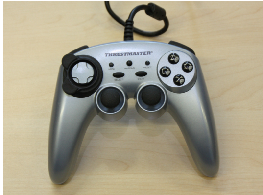
Figure 7.1: Rumble Gamepad. Both analog thumbsticks are used for moving the virtual observer, the buttons are used for various functions.
