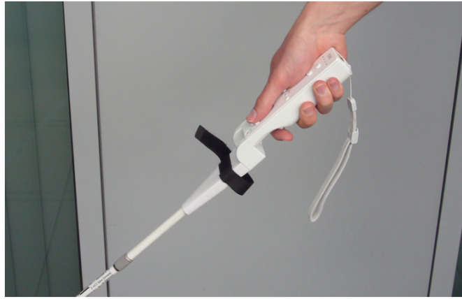
Figure 10.1: The ViibraCane. In addition to direction guidance by vibration, the cane can be used as an input device to the navigation system.
