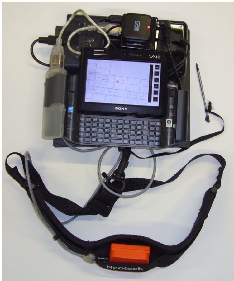
Figure 2.2: The TANIA Navigation System. The displayed map, acceleration sensor (on strap), RFID reader (left) and GPS receiver (top) can be seen.
