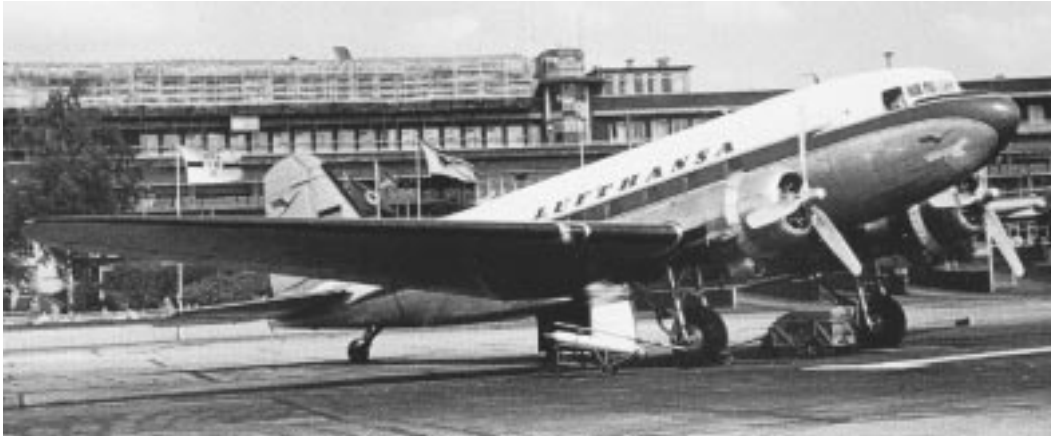
a) tail wheel landing gear configuration: DC 3
