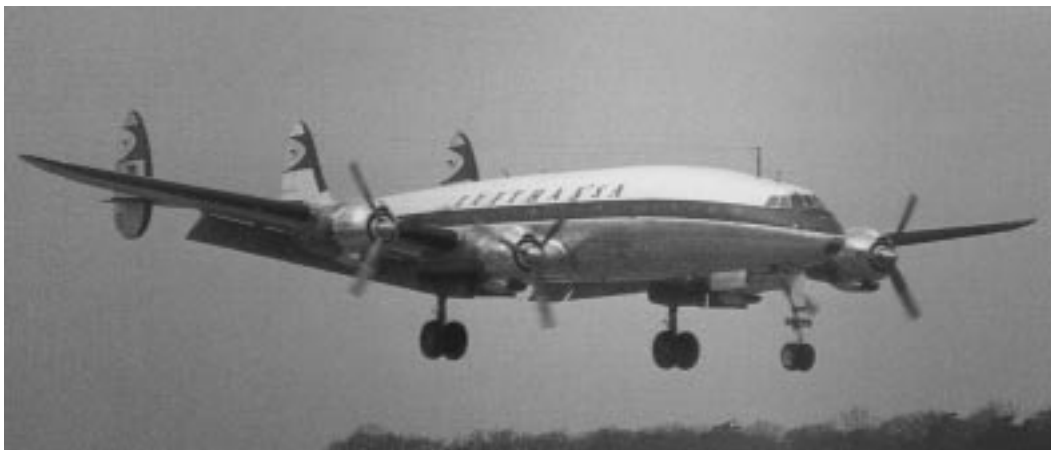
b) nose wheel tricycle landing gear configuration: L1049G
