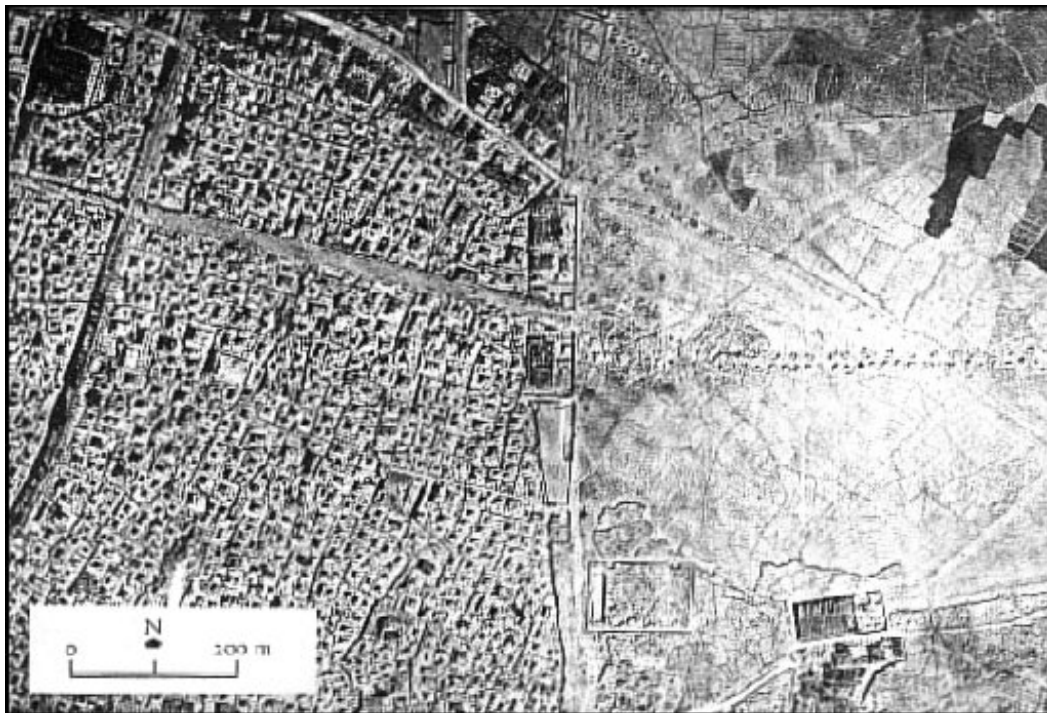
Figure 17: Qanats in Kerman city; Qanats are seen as continuous lines of mounds. Source: Kheirabadi M., 'Iranian Cities Formation and Development'.
