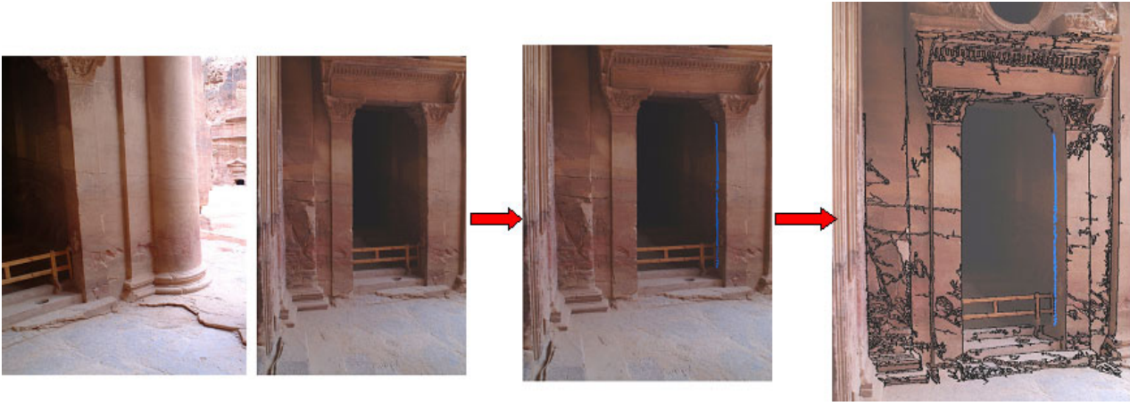
Figure 6.8: Image Based Measurements approach in order to add the inner edge to the 3D features
