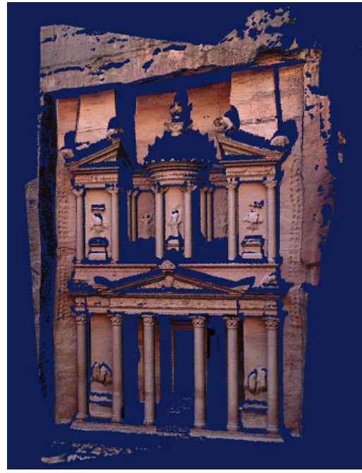
Figure 5.32: 3D Textured model using master image after separating of the occluding parts
