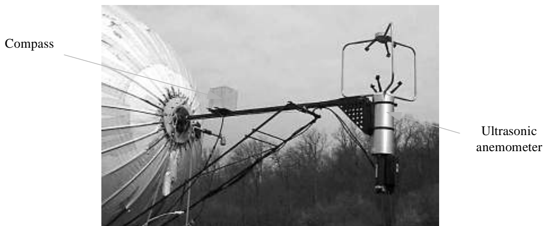
Figure 5.7: Realization of ultrasonic anemometer for airstream velocity measurements
