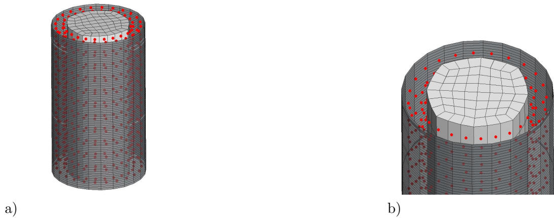
Figure 6.17: Coupled solid element/discrete particle modelling of foam filler: a) general, b) detailed view
