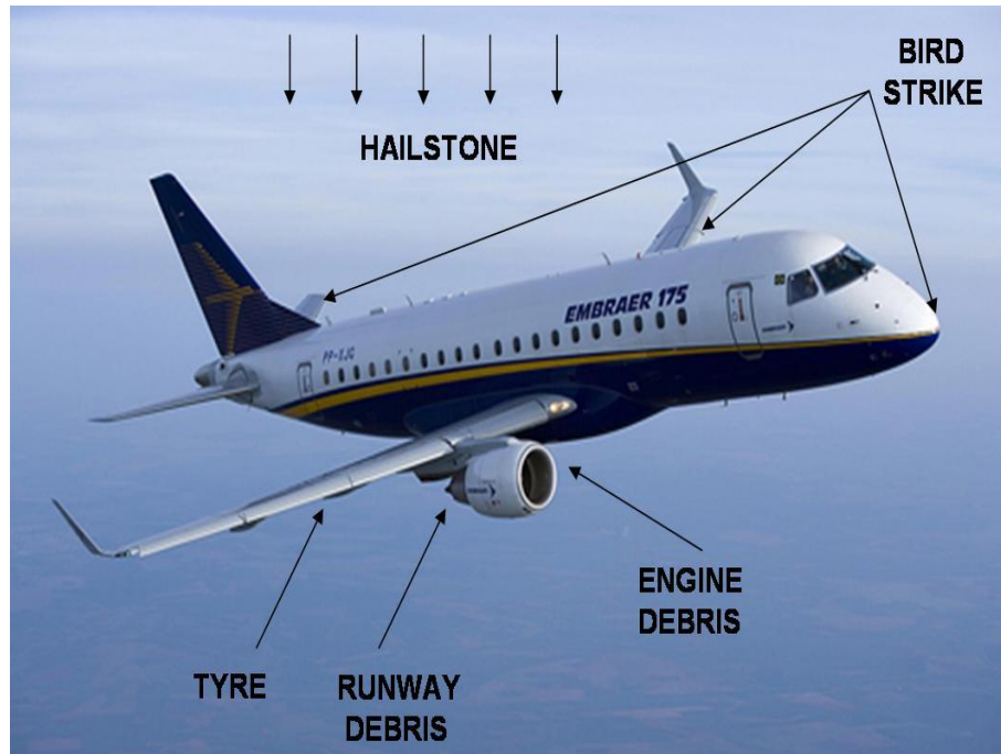
Figure 1.3: Possible impact loading cases on aircraft [3]
