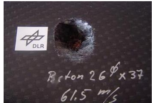
Figure 5.2: Damage to sandwich plate after impact
