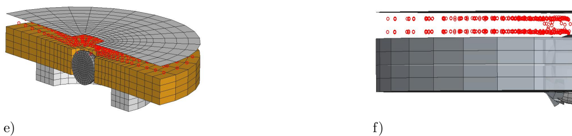
Figure 5.17: Impact states V_o = 95.1\text{m/s} : a) t=0.16\text{ms} , b) t=0.28\text{ms} , c) t=0.52\text{ms} , d) t=0.88\text{ms} , e) t=1.00\text{ms} and f) backside damage, side view
