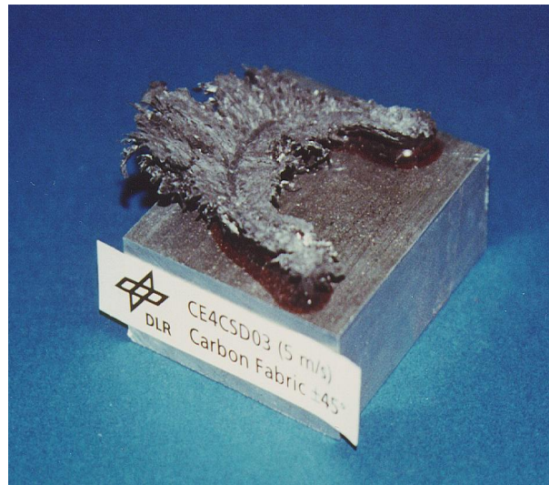
Figure 6.51: Carbon-fibre-reinforced \pm 45^\circ specimen after dynamic crushing test with v_0=5\text{m/s} [176]
