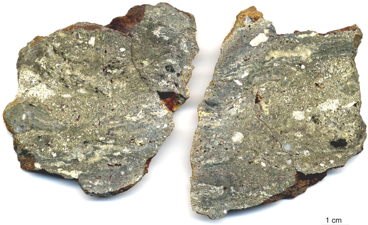
Fig. 8.4: Polished slabs of Paasselkä impact melt rocks. A distinct overall flow structure and shocked target rock components (crystalline rocks and impact-metamorphosed sandstones) are visible in the hand specimen.
