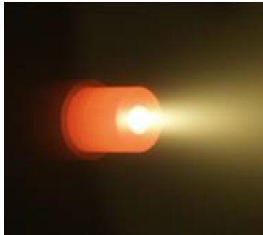
Figure 3.1: The TALOS thruster in operation[5, 48]
