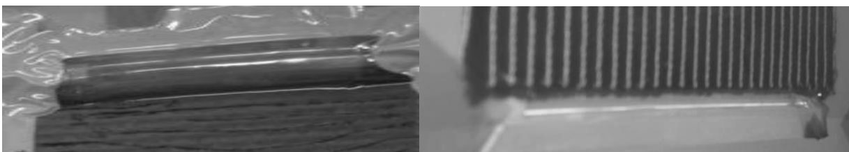
Figure 5.8 – Omega tube placement to cover the end of the fabric stack (L: top, R: bottom).
