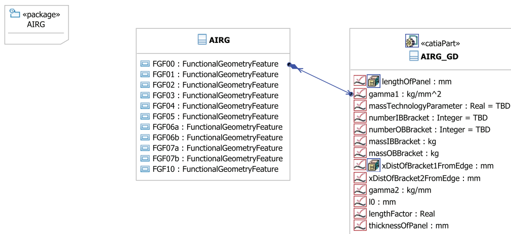
Figure C.6: The ‘air grid classes’ of the CDL_LR class diagram in UML. ‘AIRG’ inherits from ‘LRCabinModule’, ‘AIRG_GD’ inherits from ‘LRSubComponent’.
