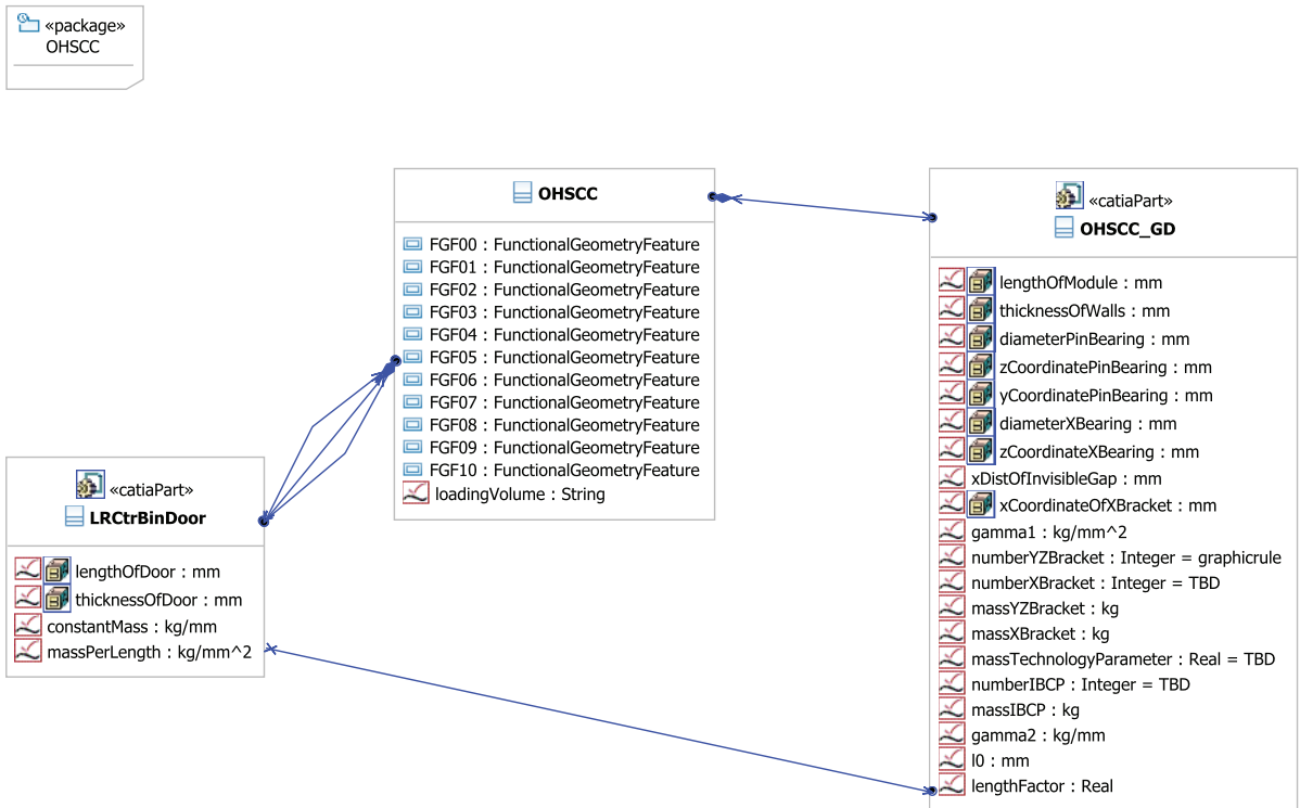
Figure C.4: The ‘center OHSC classes’ of the CDL_LR class diagram in UML. ‘OHSCC’ inherits from ‘LRCabinModule’, the others inherit from ‘LRSubComponent’.
