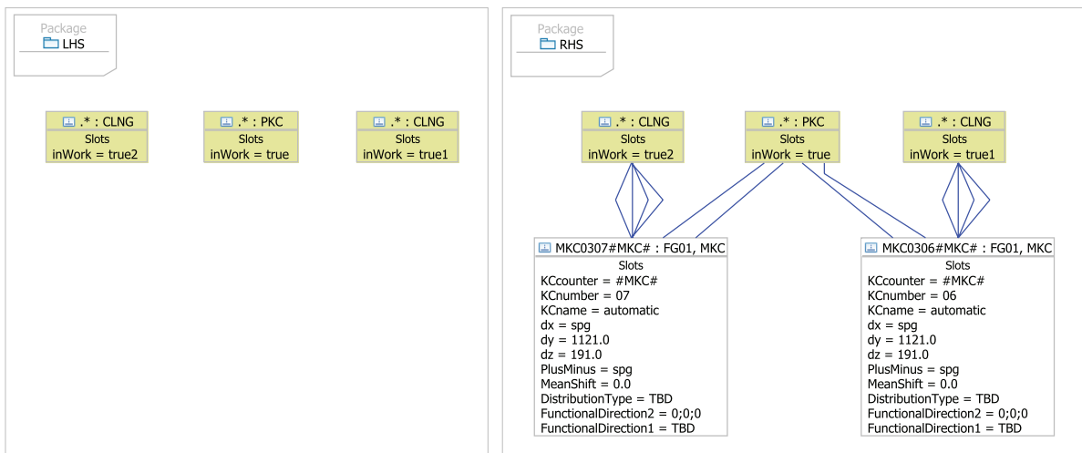
Figure 5.29: Rule 'Insert PKC001' to link a PKC instance with two ceiling panels
