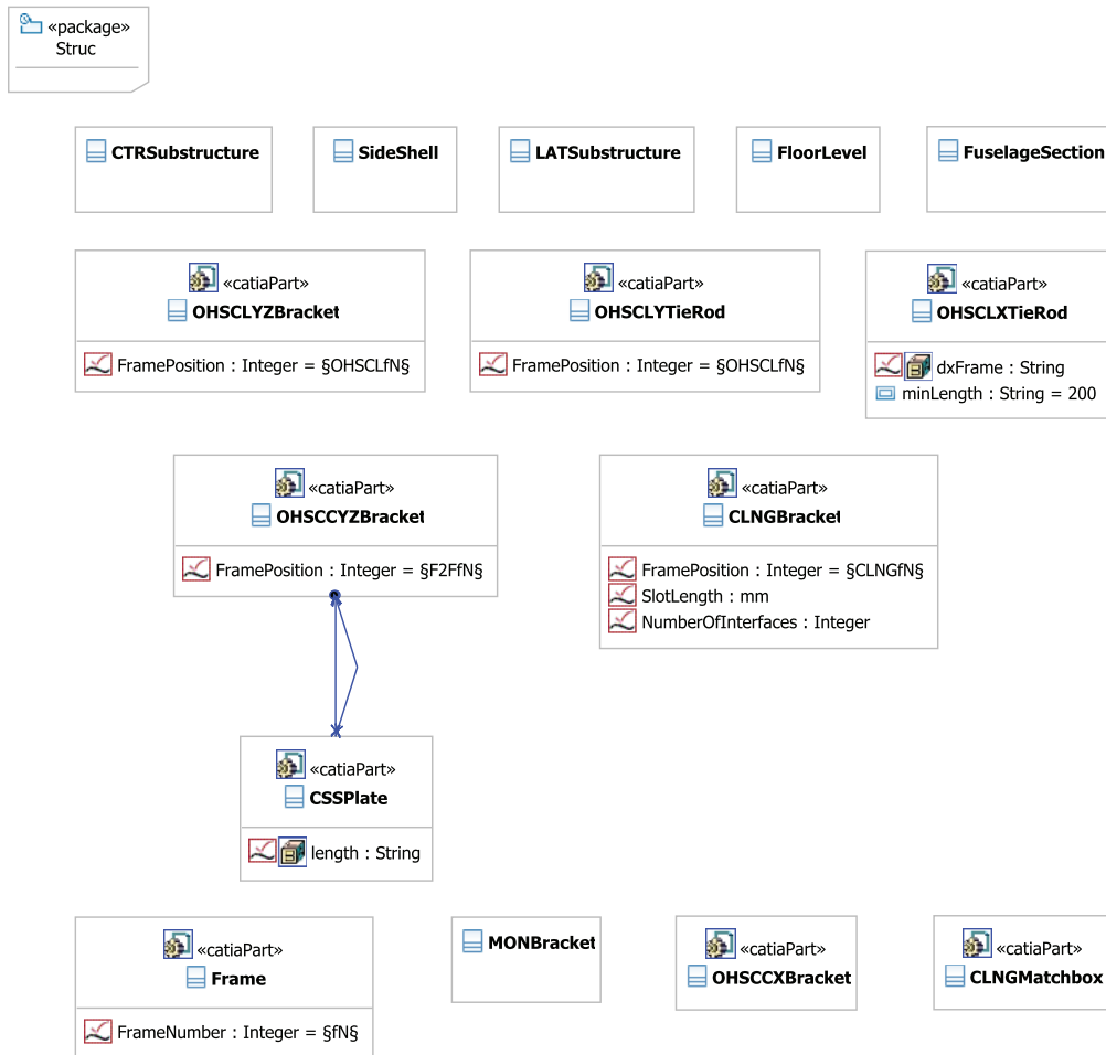
Figure C.9: The ‘aircraft structure classes’ of the CDL_LR class diagram in UML. The top five classes inherit from ‘LRStructureComponent’, the others inherit from ‘LRSubComponent’.
