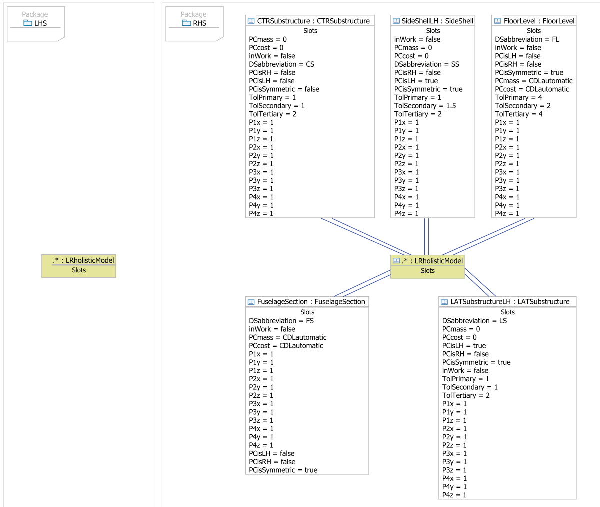
Figure 5.25: Rule 'Insert Airframe' to insert structure component instances
