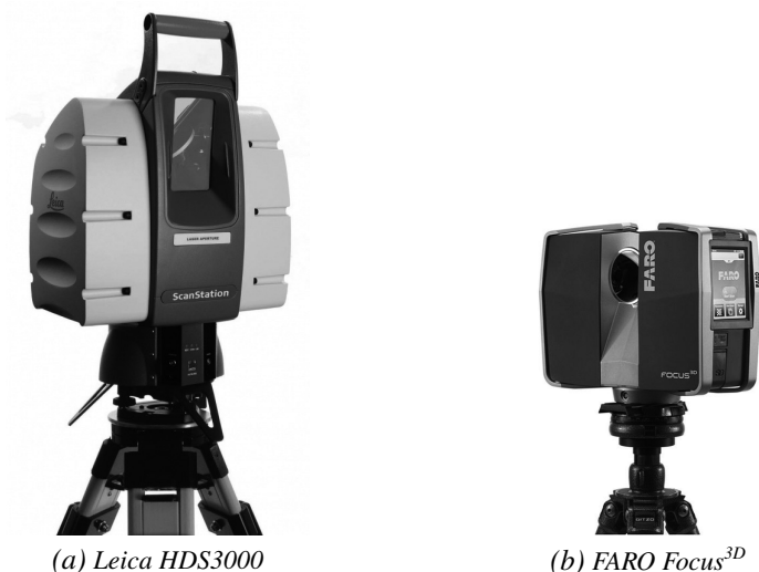
Figure 2.4: Examples of two laser scanners based on the time delay measurement principle: (a) the pulsed scanner HDS3000 and (b) the CW system Focus 3D .
