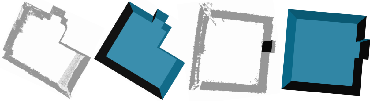
Figure 5.30: Top views of the point clouds of room A and room B with the corresponding 3D models.
