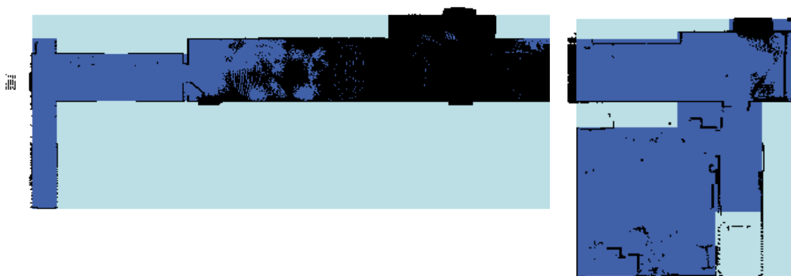
Figure 5.15: Ground plan cell decomposition results for Example C (left) and Example D (right) visualized next to each others like they are positioned in the real scene.
